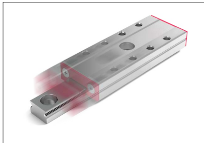
MINISLIDE MSQ allows for speeds of 3 m/s and acceleration of 300 m/s 2
